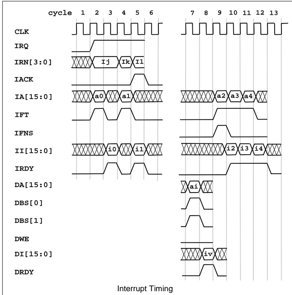
When the pipeline has been flushed the start address of the interrupt service routine is read from the interrupt vector table in data memory. **DBS[0]** and **DBS[1]** both asserted in cycle 7 (16-bit data access) with **DWE = 0** (read) indicate the reading of the interrupt vector from address *ai*. With no wait states the data access is completed in cycle 8 with **DRDY** asserted and the instruction vector *iv* available at **DI[15:0]**.
