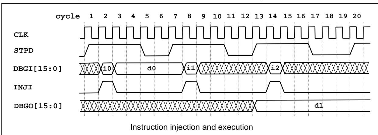
A type 2 example starts in cycle 8 where opcode **i1** is injected. When **STPD** is re-asserted in cycle 13 the destination operand **d1** is available at **DGBO[15:0]**. The example shows the behavior of an **mtdp**
