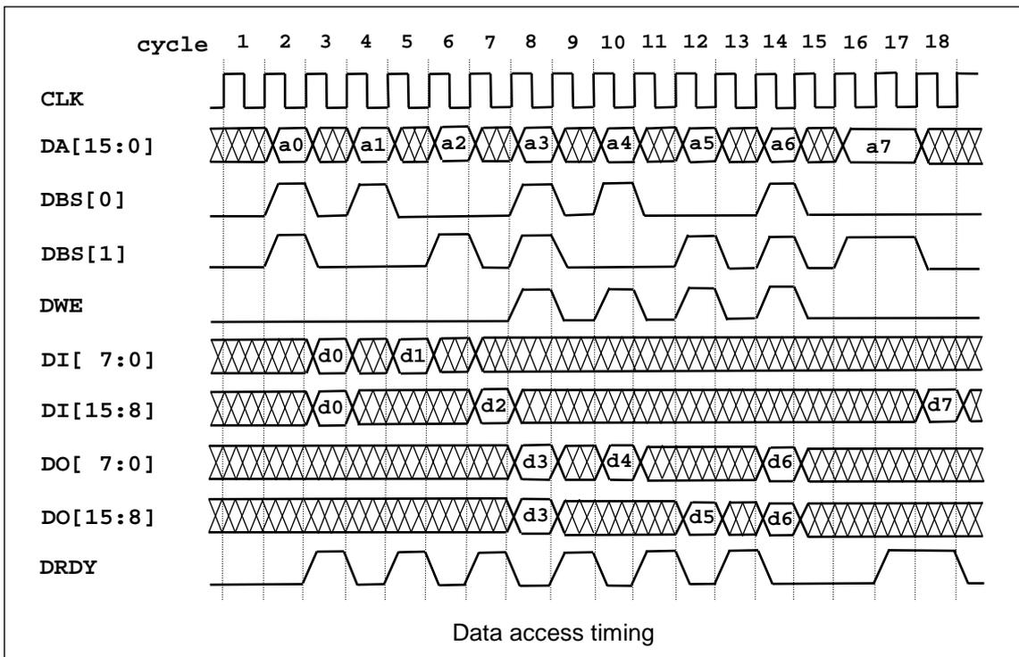
The second effect is the bus pipelining. Although the maximum access rate is one access every two cycles the bus is still pipelined as shown in cycles 17 and 18 where two accesses are completed in two consecutive cycles.
