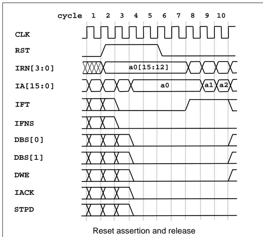
The diagram shows the `RST` assert and release timing. Only signals that are directly affected are shown. Output signals not shown are either undefined or keep their state. Beside `RST` the only input signal relevant for reset is `IRN[3:0]`.
