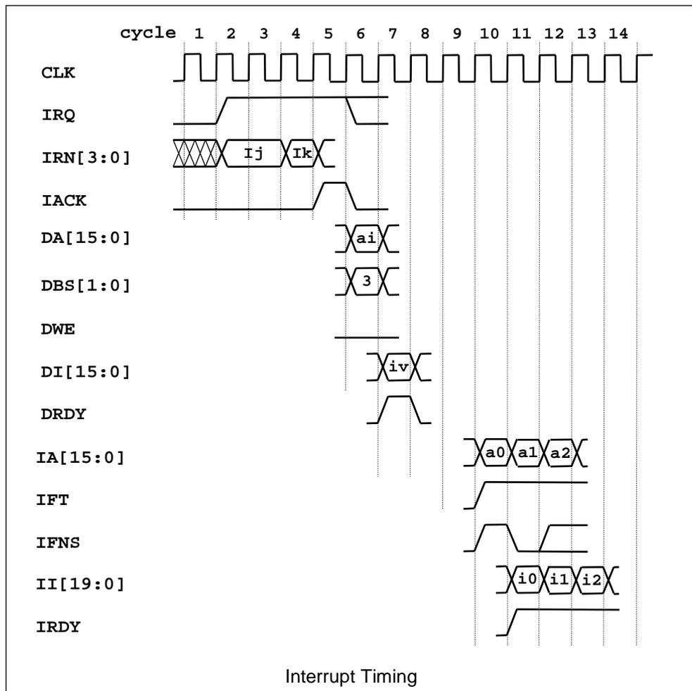
In the cycle following the  $IACK$  pulse a 16-bit data read ( $DBS[1:0] = 3, DWE = 0$ ) from address  $ai$  fetches the interrupt vector (start address).
